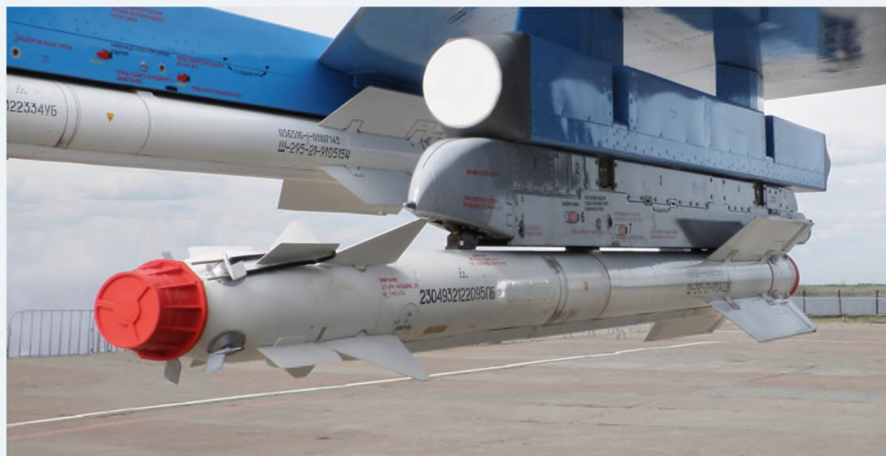
"Satellite-M2" ECM equipment onboard Su-27 and Su-30
