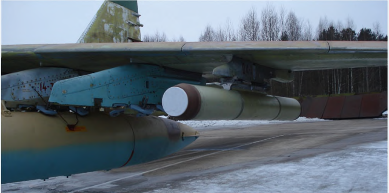
“Satellite-M2” ECM equipment onboard Su-25
