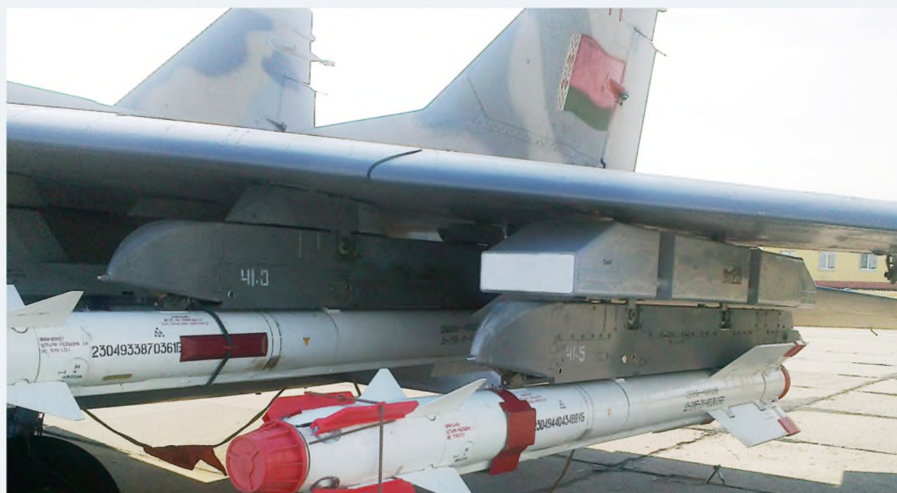
"Satellite-M2" ECM equipment onboard MiG-29
