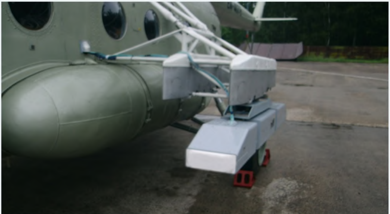
“Satellite-M2” ECM equipment onboard Mi-8 helicopter
